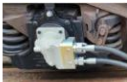
Hydraulic pump on the wheel
