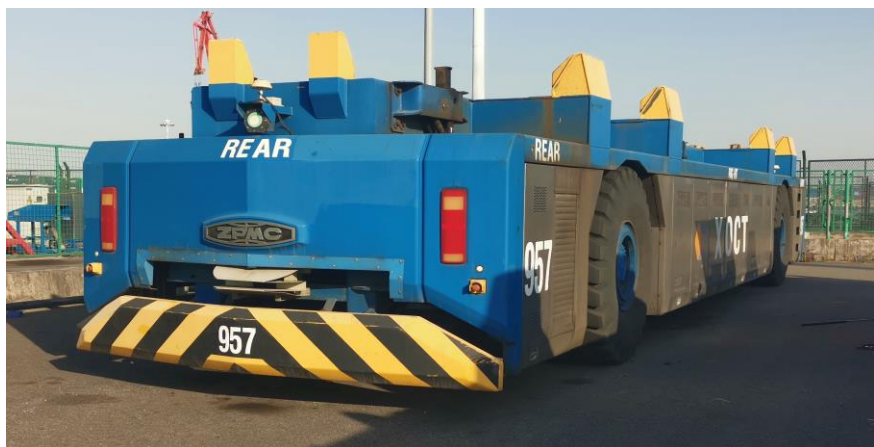
Unmanned IGV: 5 cameras (3 front + 1 rear + 1 full view)
